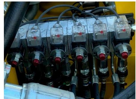
Custom Built Failsafe Manifold
